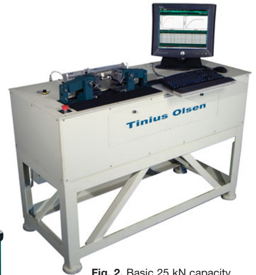
Fig. 2. Basic 25 kN capacity horizontal tensile testing machine, shown with optional extensometer
